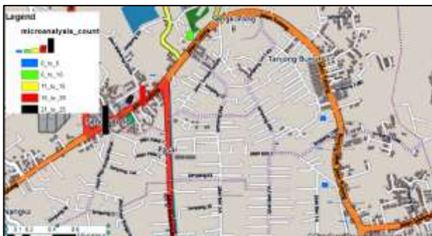
Fig. 25. Micro-analysis for road segments equal to SSD (78m).
