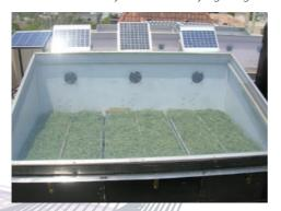
Brief explanation: Solar dryers are devices that use solar energy to dry substances, especially food. Open-air, sun drying of agricultural products is the traditional method employed in most of the developing countries. Sun drying is used to denote the exposure of a commodity to direct solar radiation and the convective power of the natural wind. This technology helpful for the agriculture industry in Brunei.
